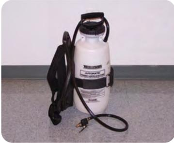
Heavy-duty plunger with chemically resistant Viton seals for long-life dependability. Finger Touch Control Valve allows the operator to easily control the amount of finish dispensed through the honey-combed fiberglass handle into either of the two applicator heads.
